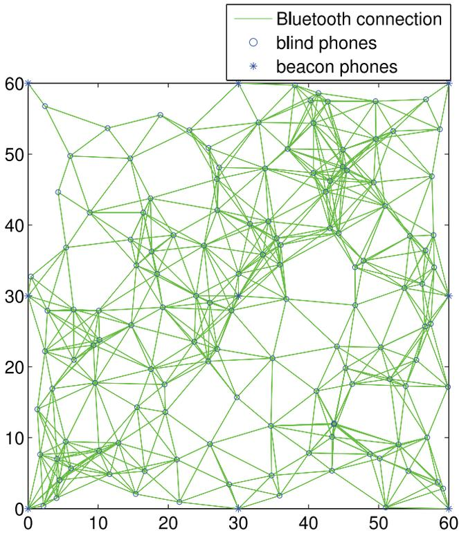
Fig. 8. True positions of phones in the Bluetooth network and the Bluetooth connection topology in the supermarket localization application.
