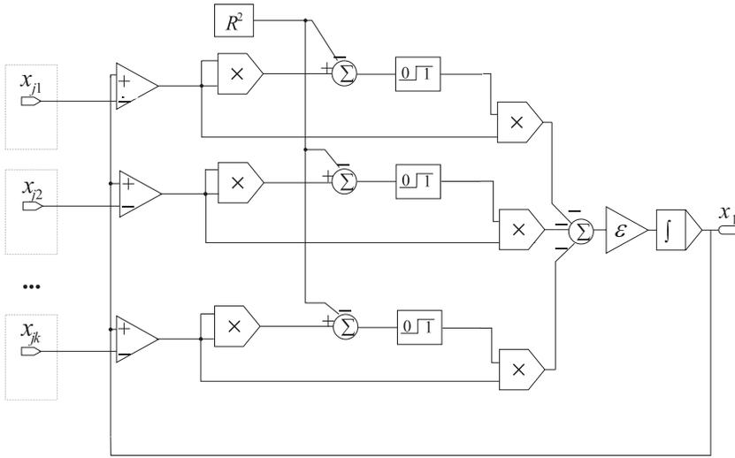
Fig. 2. Analog circuit architecture of a module in the proposed neural network.
