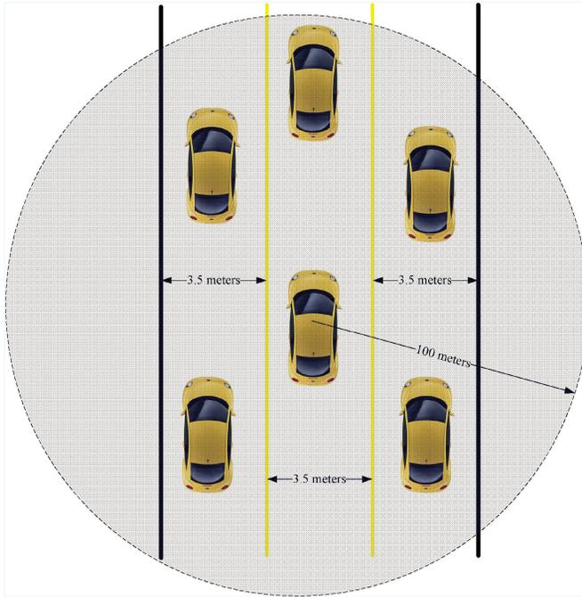
Fig. 4. The sketch of the Bluetooth aided localization in a tunnel.
