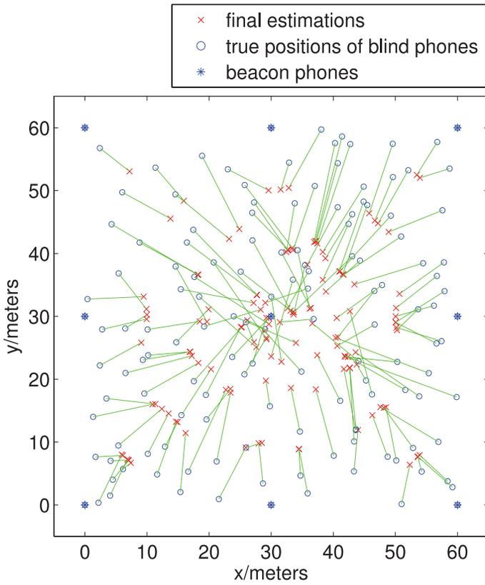
Fig. 9. Position estimation results in the supermarket localization application.
