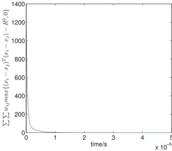
Fig. 12. Time evolution of  $\sum_i \sum_j \max\{(x_i - x_j)^T(x_i - x_j) - R^2, 0\}$  in the supermarket localization application.
