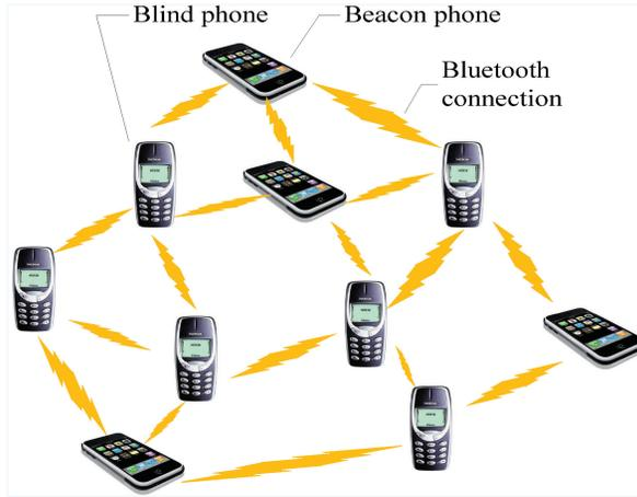
Fig. 1. Connectivity topology of the Bluetooth aided mobile phone localization system.
